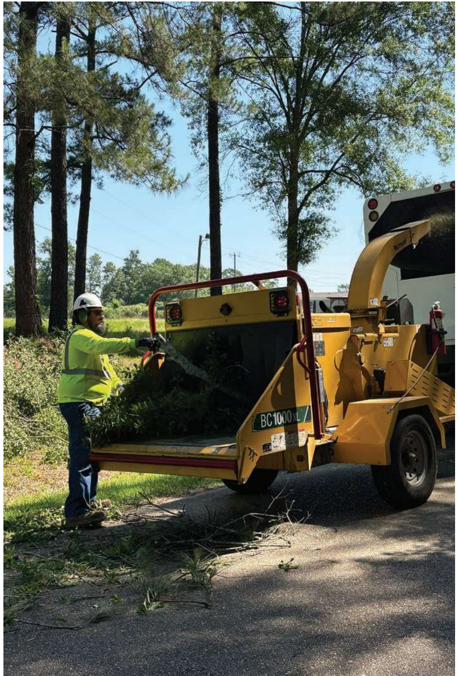
ABOVE: Tree limbs are loaded into a chipper after right-of-way tree trimming.
