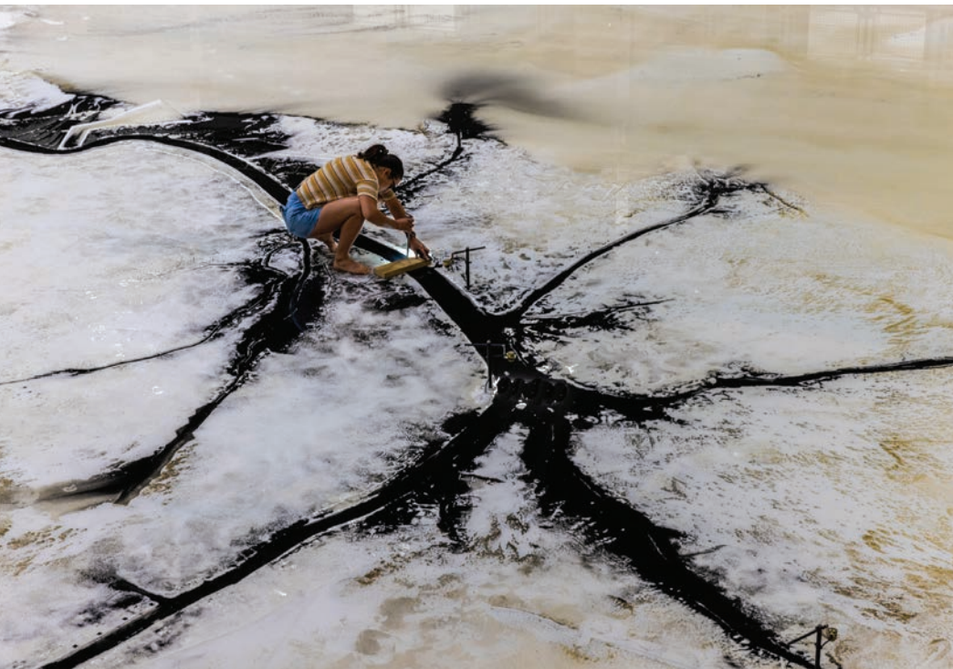
A student researcher measures changes in sediment load and dispersion using a physical model the size of two basketball courts.
