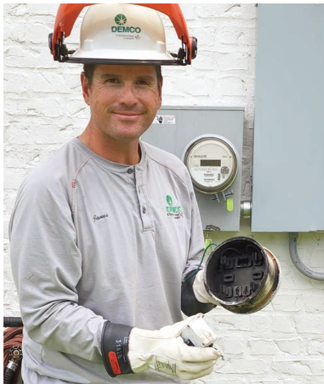
DEMCO’s James Macias holds a meter device damaged by a voltage surge from a nearby lightning strike. The meter-based surge protector prevented the surge from entering the home. The member reported no items damaged at the location.
